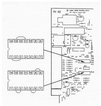
Figure C-1 TTL Header Installation Diagram.
